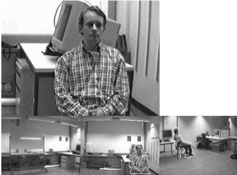
Fig. 3. Zoomed-in image of the segmented object is shown on the top, small images on the bottom line show available views and extracted silhouettes in them.
