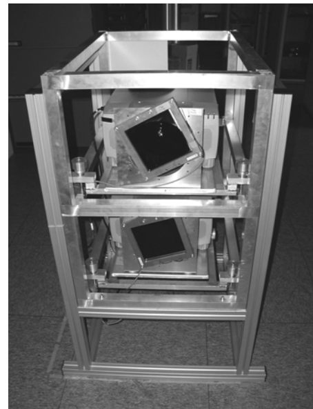
Figure 4. Stereo projection rack with LC-shutters
