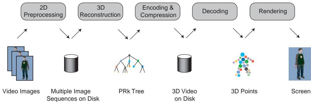
**Figure 1:** System Architecture of the 3D Video Recorder. The pipeline illustrates the process for one frame.
