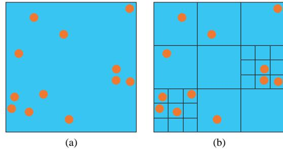
**Figure 3:** An example of a 2D two-level PR9-tree ( $s=3$ ). Each node is decomposed into nine child nodes. (a) Distribution of points in the plane at level zero. (b) Decomposition of the PR9-tree at level two.
