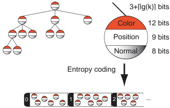
Figure 4: Overview of the PRk tree encoding.
