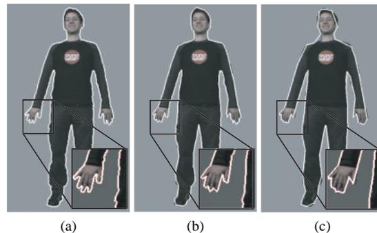
**Figure 2:** Different scales in the contour extraction. (a) An exact contour with 2548 points, (b) an approximation with 221 points (threshold=5), and (c) an approximation with 94 points (threshold=15).
