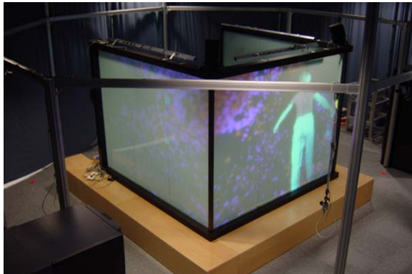
Figure 8: The blue-c: An immersive telepresence installation allowing simultaneous acquisition and projection.
