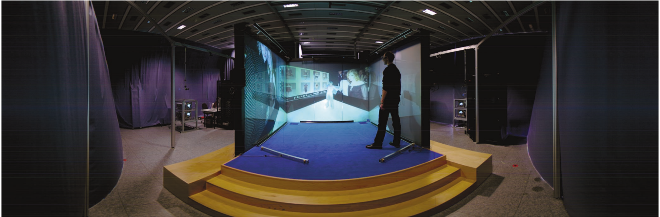
Figure 1: Panoramic picture of the blue-c portal showing the projection screens in transparent mode, the outer scaffold with attached cameras, the LED arrays, and the LCD stereo projectors.
